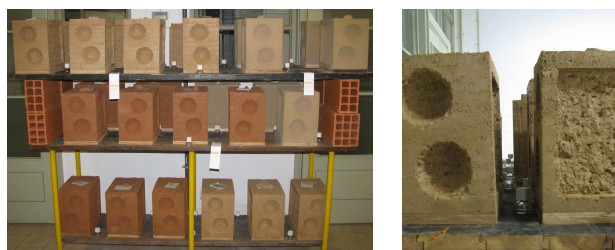
Figure 2. Rammed earth laboratory blocks with different soils and with two types of surface degradation - deep voids and superficial irregularity with loss of cohesion.
