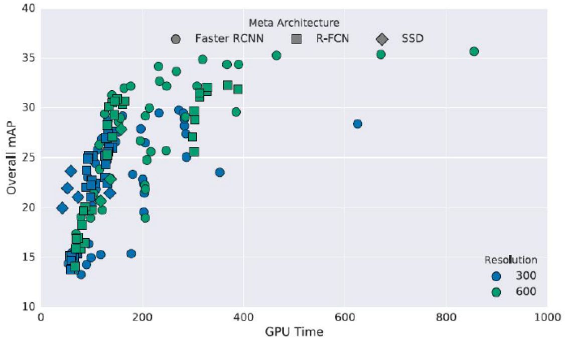
Figure 3.2: Effect of image resolution in the overall mAP using different meta-architectures [20]
