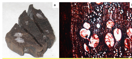
Fig. 5 – Quercus sp. (7) timber sample (a); cross section observed under the microscope (b); scale = 400µm.
