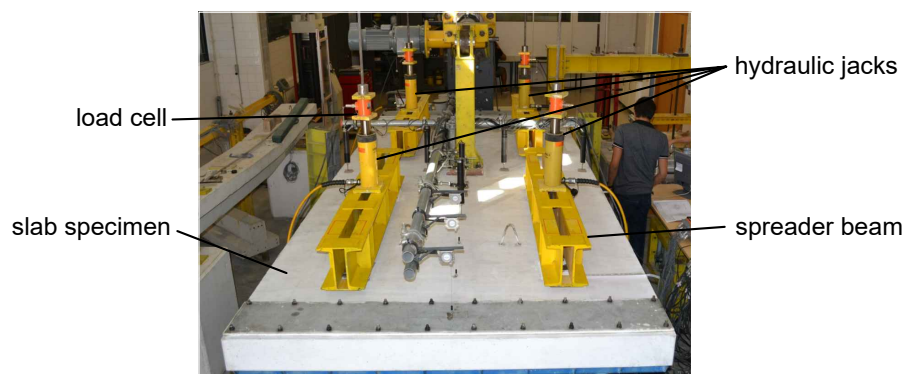
Figure 3.19: Gravity load application
