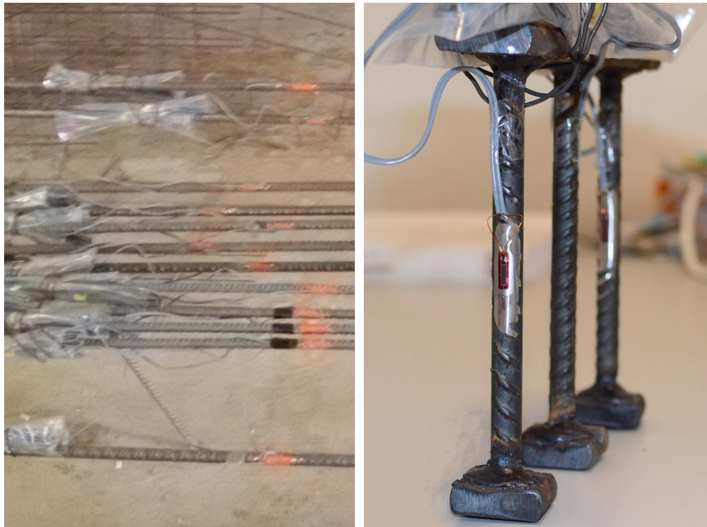
(a) Strain gauges in longitudinal bars
