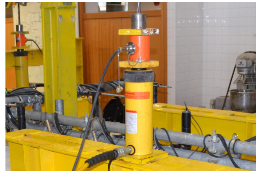
(b) Hydraulic cylinder and load cell for gravity loading
