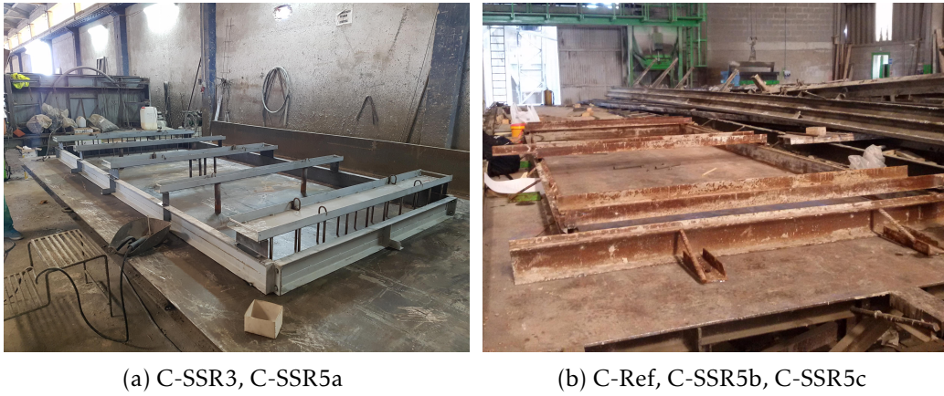
Figure 3.12: Moulds used to cast the specimens
