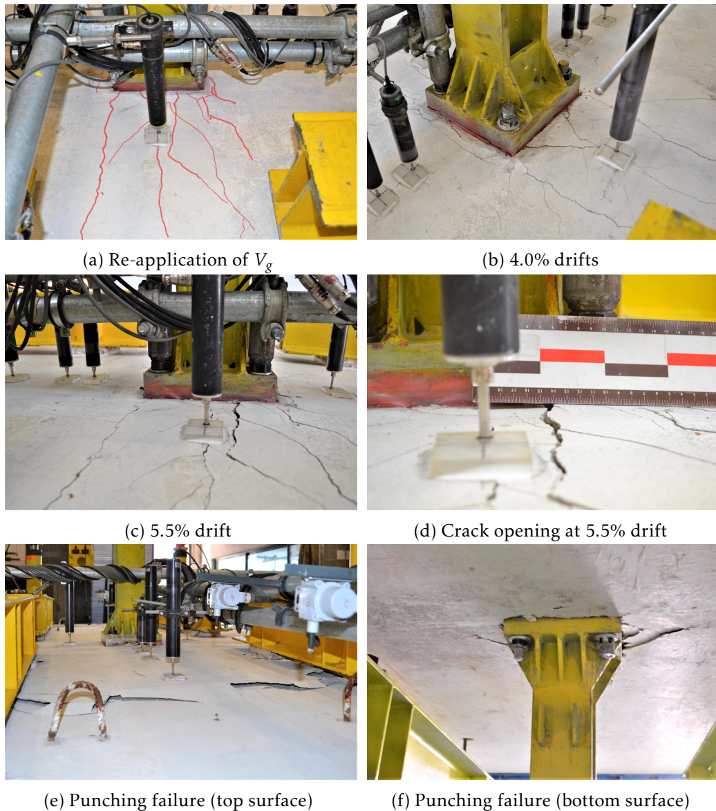
Figure 3.33: Photos during the second phase of cyclic loading test of specimen C-SSR5b
