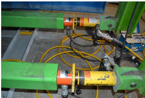
(c) Hydraulic cylinders and load cells in the test setup struts
