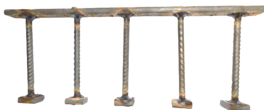
(b) A stud rail for specimens C-SSR5(a, b, c)
