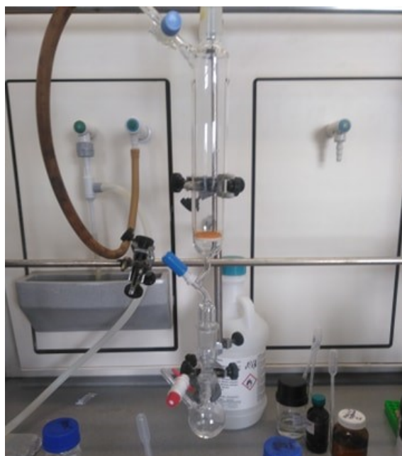
Figure 2.1: SPPS assembly, consisting on a filter reaction vessel, round bottom flask, neck glass adapter and a nitrogen stream.
