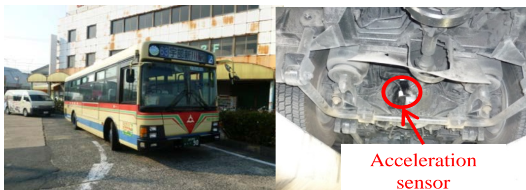
Figure 5 Fixed-route bus and sensor used for long-term field testing
