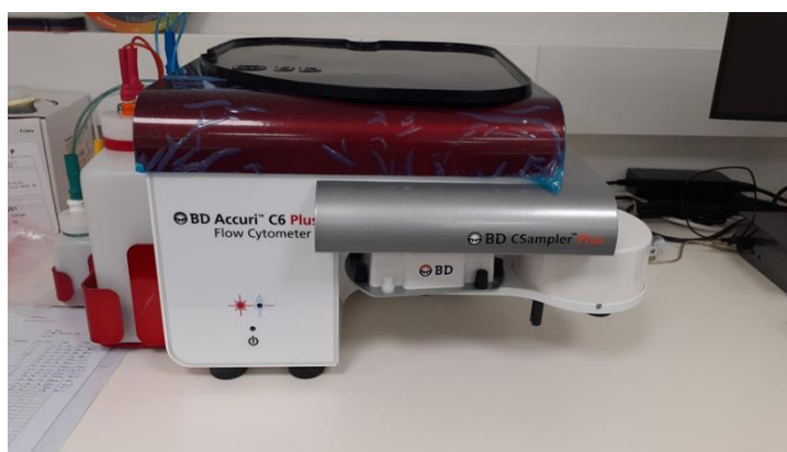
Figure 3.4 - BD Accuri™ C6 Plus Flow Cytometer used for rate of infection determination
