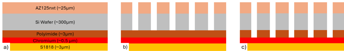
Figure 19 – Single polyimide chromium sample expected evolution; a) expected design after wafer processing; b) expected result after DRIE; c) expected result after RIE
