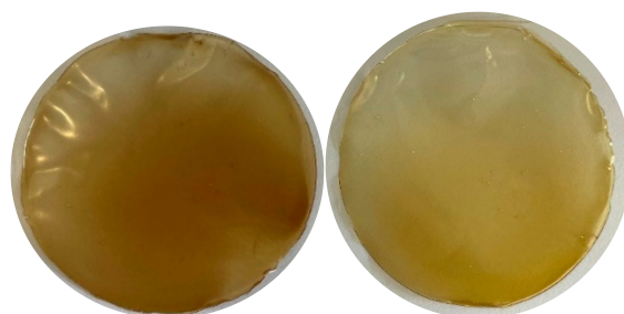
Figure 7. Formulated arabinoxylan film without resin contact (Ax, left) and after resin contact (AxR, right).
