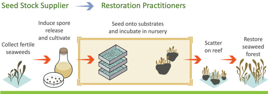
Figure 2 - Cross-sectoral approach to marine forest restoration - Cultivation of green gravel Source: SeaForester 2024
