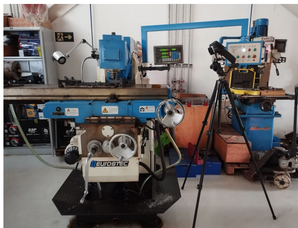
Figure 2 – Final assembly of the thermographic camera for data acquisition: positioned along the direction of the welding tool
