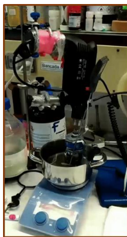
Figure 5 – Photo of the stirred vessel built for small scale extractions of suberin with the ionic liquid approach.
