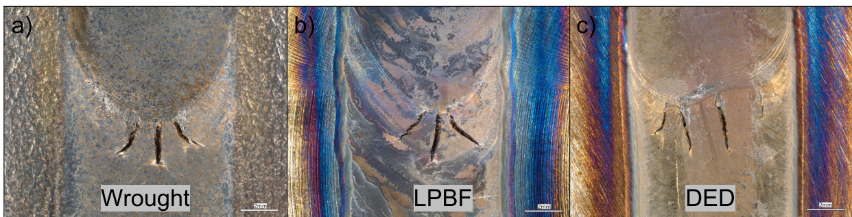
Fig. 7. Alloy 718 cracking at 3 % strain. a) Wrought, b) LPBF, and c) DED.
