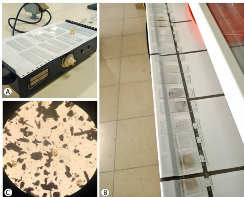
Figure 3.9 — The slides preparation for microscopic observation: a) Coverslips and thin sections placed on the heating plate along with melted glycerinated gelatine suppositories used to seal them; b) Slides drying post-placement of palynological residues and coverslips; c) Photographic documentation of an analysed slide revealing palynomorphs.
