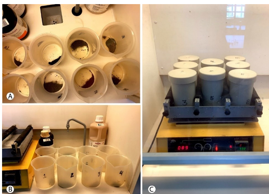
Figure 3.8 — Palynological treatment processes: a-b) The fractioned outcrop samples, 30 g per container, before the hydrochloric acid (HCl 37%) treatment; c) Samples in Teflon containers following the second acid treatment with hydrofluoric acid (HF 48%) to dissolve silicates, agitating on an orbital shaker.
