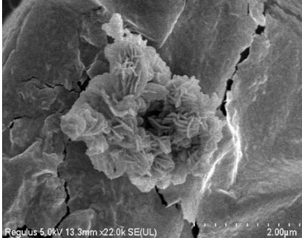
D - SEM image of a MXene in GelMA+MX+LAP
