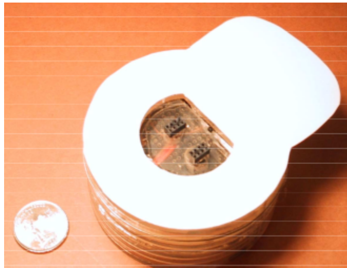
Figure 2.18: A Sensetable puck, with a socket for attaching a dial or modifier. A US quarter is shown for scale [51]
