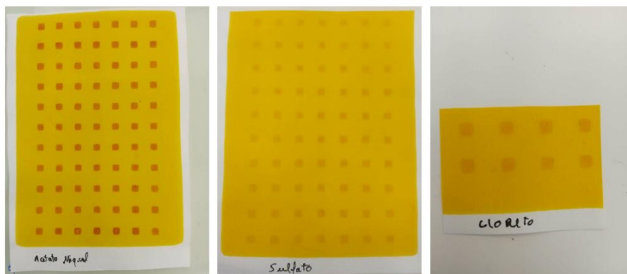
Figure 3.4 — Different nickel precursors used with the drop cast technique (nickel acetate, nickel sulfate and nickel chloride). All samples present 0.5 \mu\text{l}/\text{mm}^2 ratio.
