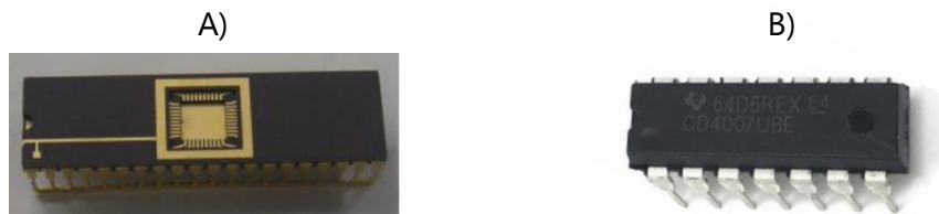
Figure 4.3: Used MOSFETs; A) Packaging of the developed MKProt; B) Commercial MOSFET CD4007UB by Texas Instruments
