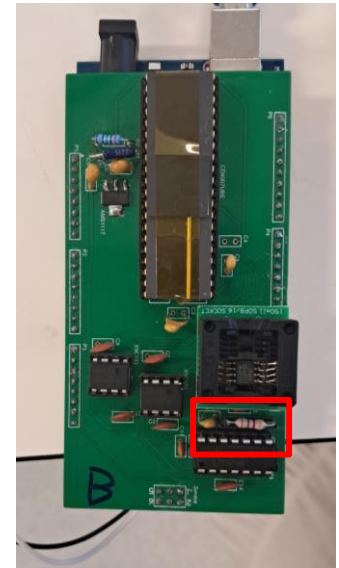
Figure 5.4: Custom-PCB; A) Schematic diagram; B) PCB with changeable resistor marked in red rectangle.
