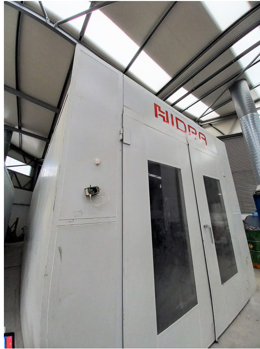
Figure 4.22: Sensor Box attached to a painting booth. And close to the corresponding beacon.
