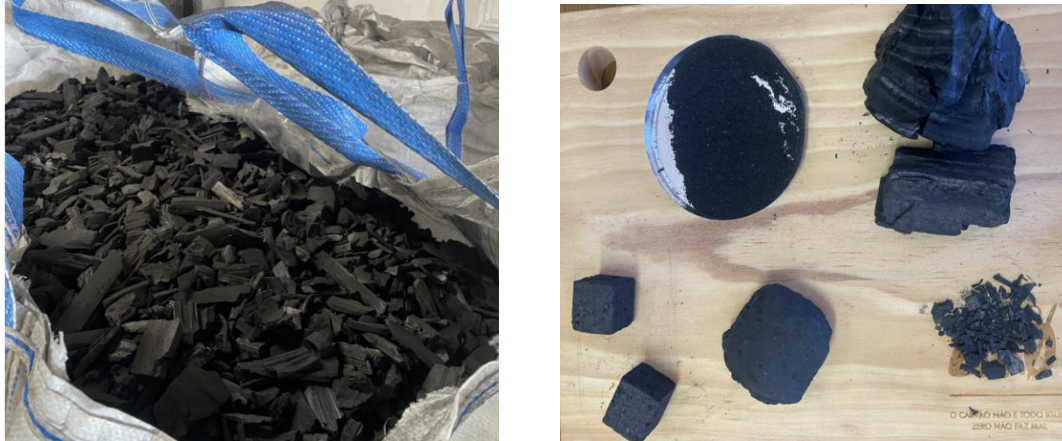
Figure 1: Biochar in bulk (left); Forms of biochar - from powder to coal (right); Pictures taken at Ibero Massa Florestal
