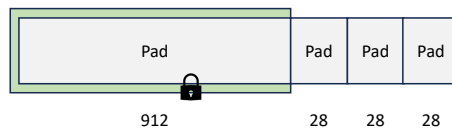
Figure 4.23: Response Packet for the Entry Node Key Exchange.
