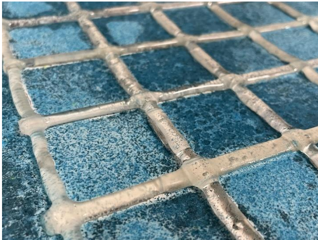
Figure 68 Clayze applied onto sheet of window glass, and strips of glass added on top and fired. Revealing the coarse body of a fired Egyptian paste trapped between the glass, while showing the colored surface on the rest of the glass sheet. (©Nour Ali)
