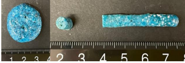
Figure 40 Recipe H at 950 °C, (left) cross section (right) (©Nour Ali)
