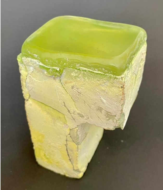
Figure 69 Glass casting into mold lined with clayze. (©Nour Ali)
