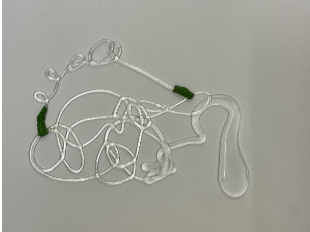
Figure 67 Coils of Clayze mixture used to glue two pieces of glass together. (©Nour Ali)
