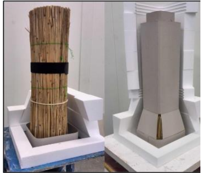
Figure 19 Core used to make the pillar (Tajeddin, 2014)
