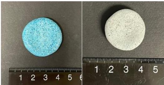
Figure 47 Recipe A at 840 °C (left) and 750 °C (right) (©Nour Ali)
