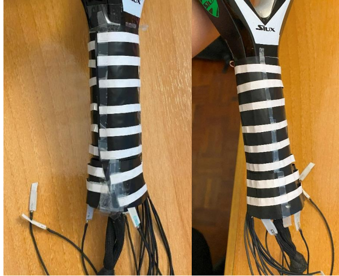
Figure 5.6 – State of the paper with Velostat grip after testing.
