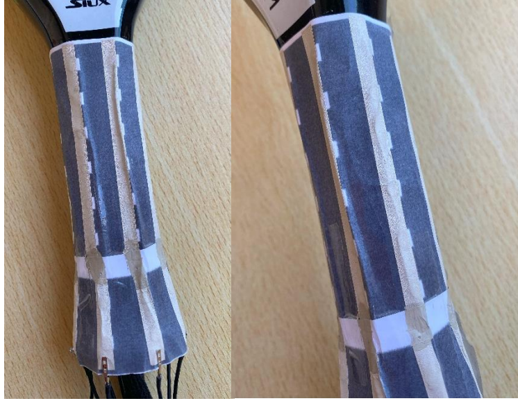
Figure 5.8 – State of the paper with hydrogel grip after testing.
