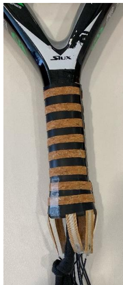
Figure 5.7- State of the cork with Velostat grip after testing.
