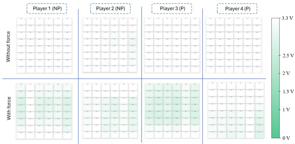
Figure 3.17 - Players performance with the cork with Velostat grip with a R_{bias} of 330 \Omega during player-interface evaluation.
