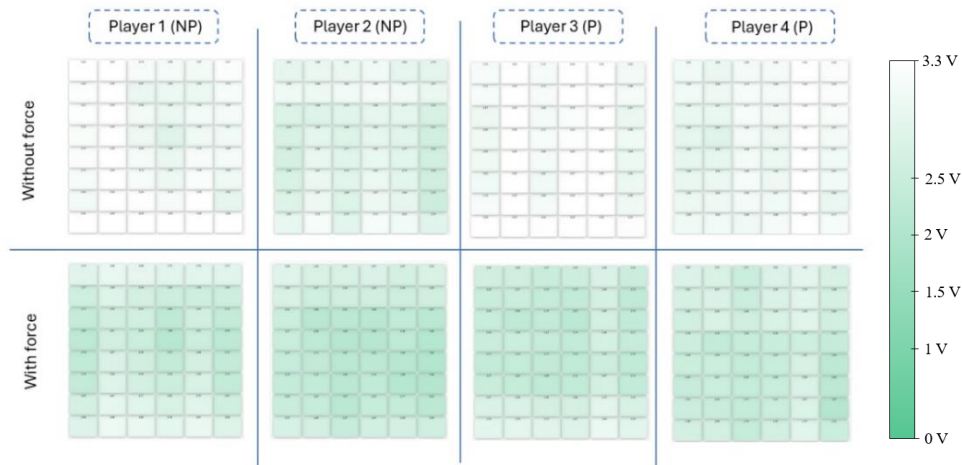
Figure 3.22 - Players performance with the cork with Velostat grip with a R_{bias} of 1 \text{ k}\Omega during player-interface evaluation.
