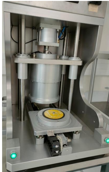
Figure 16: Mechanical press to enhance the bonding of the closing tape.
