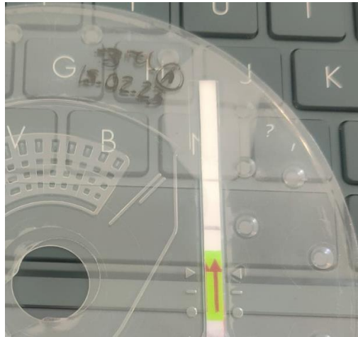
Figure 45: LFA strip interfering with the bonding of the closing tape.
