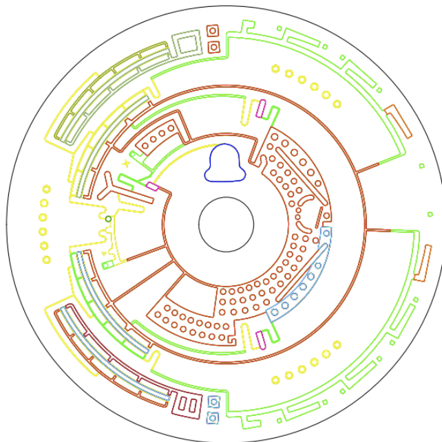
Figure 21: Microfluidic layout from the CRP disc obtained from biosurfit , detection chambers are located on the right side of the disc and highlighted in green (further explanation of the layout is available in the supplementary material).
