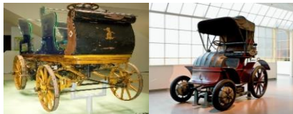
Fig. 2: (Left) Egger-Lohner C.2 Phaeton, Porsche's first contribution. (Right) Lohner-Porsche Electromobile, designed by Porsche, first hybrid-electric car Sources: Flickr, Supercars.net
