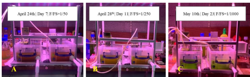
Figure 3.15- Reactor A and Reactor B at 3 different days, under three different F/FS ratios: A-1/50, B-1/250, C-1/1000.
