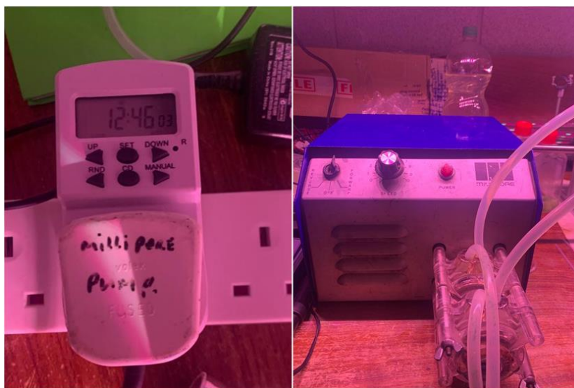
Figure 3.13 - Digital timer used for the pump (Left) and Peristaltic Pump (Right)
