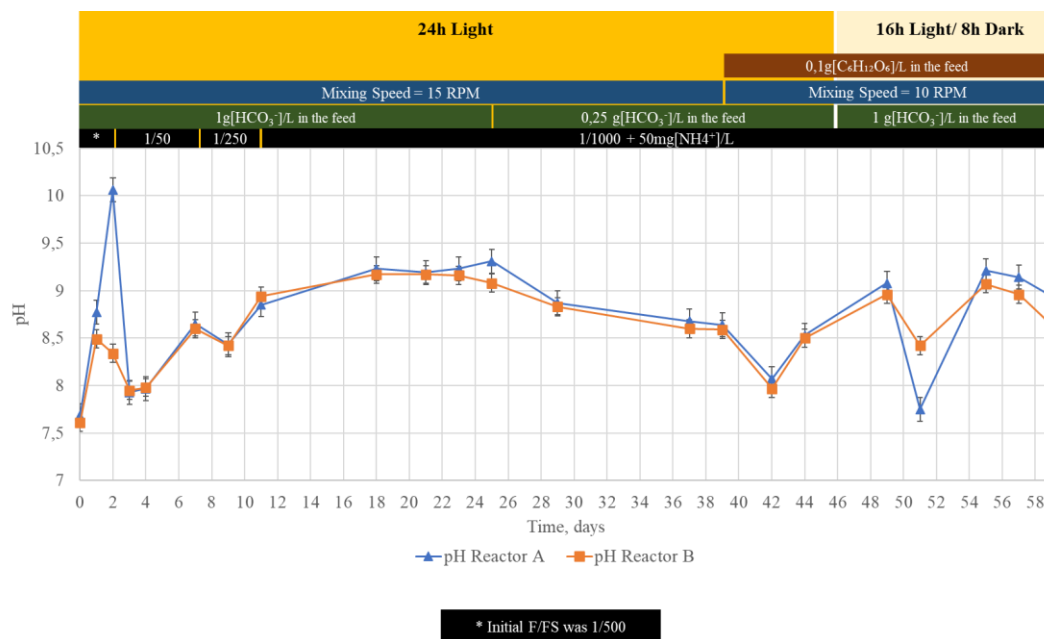
Figure 4.2 - pH progression in Reactor A and B during the 1st Stage. F/FS - Fertiliser/Feed Solution; Black bars represent the different F/FS ratios implemented
