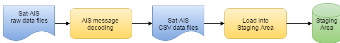
Figure 5-1 – Sat-AIS data processing chain
