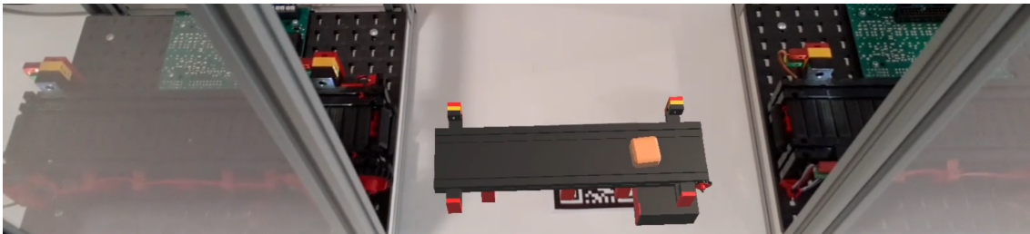
Figure 5.2: Conveyor arrangement with the Virtual Conveyor positioned between the Physical Conveyors in operation.
