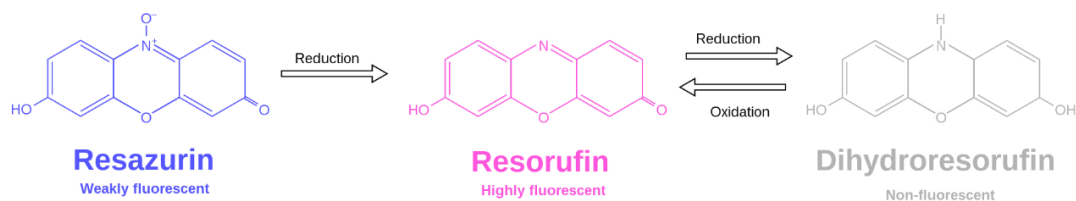
Figure 2.2 – Redox reactions undergone by resazurin. Resazurin shows a blue color, resorufin a pink color, and dihydroresorufin is colorless. The reaction from resazurin to resorufin is irreversible, while the reaction from resorufin to dihydroresorufin is reversible and only happens at -110 mV (reduction reaction).
