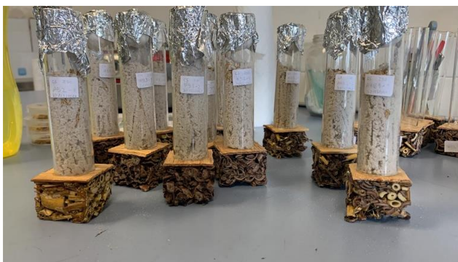
Figure 5.5-2. Samples to evaluate the resistance to termites according to an adaptation of EN 118 (EN 118, 2013) with the glass tube glued to the wooden boards.
