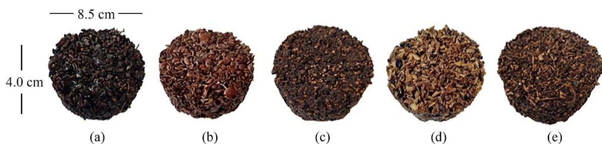
Figure 3.3-3. Samples B – sodium silicate solution: (a) grape press waste (BG); (b) hazelnut shells (BH); (c) olive press waste (BO); (d) wood chips (BW); (e) wood chips and spent coffee grounds (BWc).
