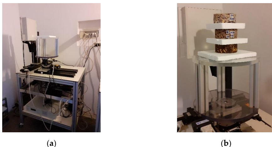
Figure 5.2-3. X-ray computed tomography: (a) employed apparatus; (b) three samples separated by expanded polystyrene boards placed on the rotation platform.
