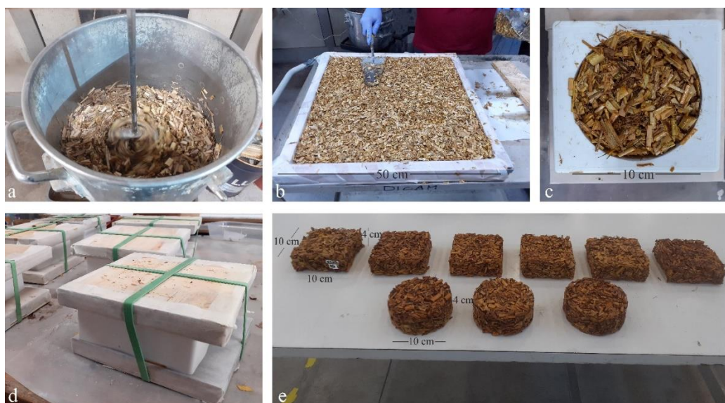
Figure 4.4-2. Some steps of the production process of composite samples made of giant reed and the sodium silicate solution: a) mechanical mixing of the aggregates and the adhesive; b) moulding (wooden mould 50 cm x 50 cm x 4 cm) by using a spatula; c) cylindrical mould (diameter = 10 cm, high = 4 cm) with the mixture of giant reed and sodium silicate solution; d) closed moulds (10 cm x 10 cm x 4 cm); e) rectangular and cylindrical composite samples after demoulding and curing phase.
