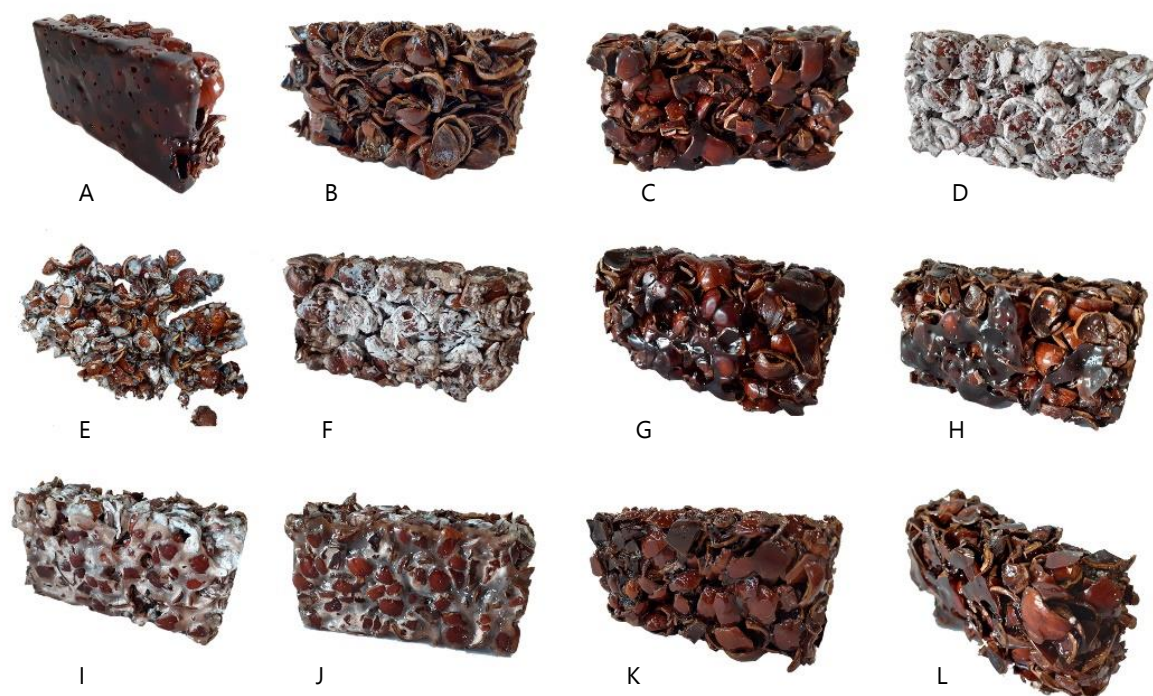
Figure 4.2-4. Representative composite samples produced by using different production parameters after demoulding, from A to L.
