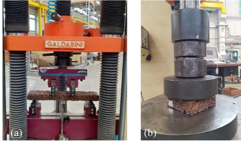
Figure 4.3-7. Galdabini universal machine employed to evaluate the mechanical properties: (a) sample 10 cm x 50 cm x 4 cm used to analyse the flexural strength; (b) sample 10 cm x 10 cm x 4 cm used to evaluate the compressive strength.
