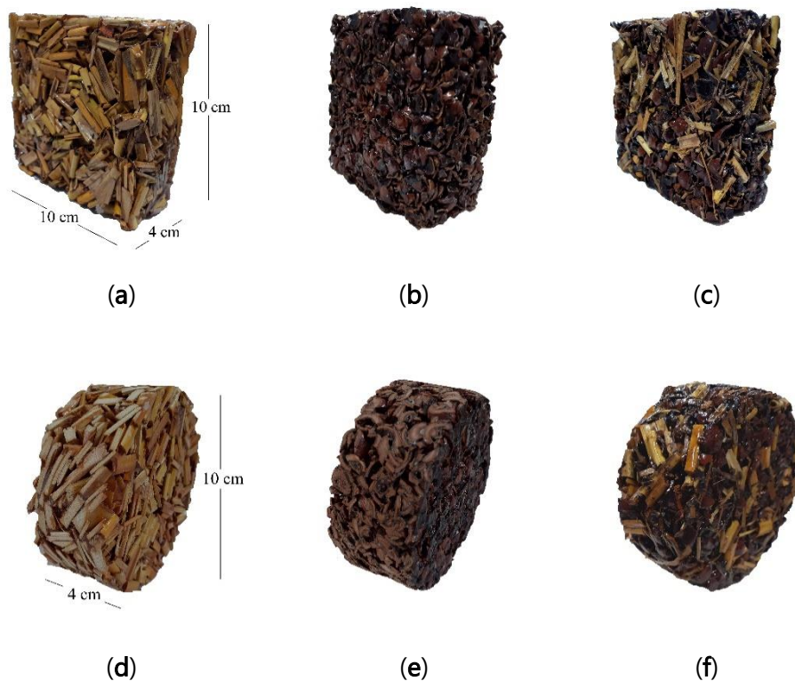
Figure 5.2-2 Composite samples made of bio-aggregates and sodium silicate solution. Rectangular and cylindrical samples: (a,d) A. donax -based composite—A; (b,e) hazelnut-shell-based composite—H; and (c,f) A. donax + hazelnut-shell-based composite—AH.
