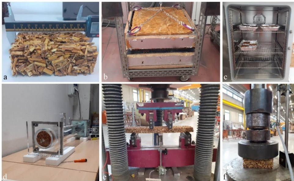
Figure 4.4-3. Main tests of the experimental campaign: a) evaluation of the apparent density of a giant reed-based composite sample; b) equipment to evaluate the thermal conductivity by the heat flow method; c) composite samples into the climate chamber during the hygroscopicity test; d) a cylindrical sample of giant reed into the impedance tube to evaluate the sound absorption capacity; e) giant reed-based sample (10 cm x 50 cm x 4 cm) in the Galdabini machine at the beginning of the bending test; f) giant reed-based sample (10 cm x 10 cm x 4 cm) before the performance of the compressive test.
