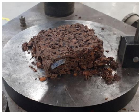
Figure 4.3-13. Rectangular sample of hazelnut shells and sodium silicate solution after the compressive test and the achievement of the breaking load.
