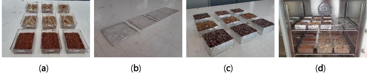
Figure 5.2-4. Samples for the hygroscopicity test: (a) plastic boxes (15 cm × 11 cm) filled up to 2 cm with the different aggregates (samples AA, HH, and AAHH); (b) air-dried sodium silicate solution covered with aluminum foil, except for the exposure surface (area = 0.1 m 2 ); (c) composite samples (aggregates + sodium silicate solution) A, H, and AH (10 cm × 10 cm × 4 cm) covered with aluminum foil, except for the exposure surface (area = 0.1 m 2 ); and (d) samples in the climatic chamber.
