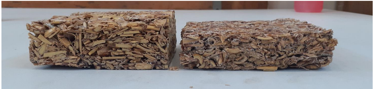
Figure 4.4-10. Example of two giant reed-based composite samples employed for the compressive test before (left) and after the compressive test (right).
