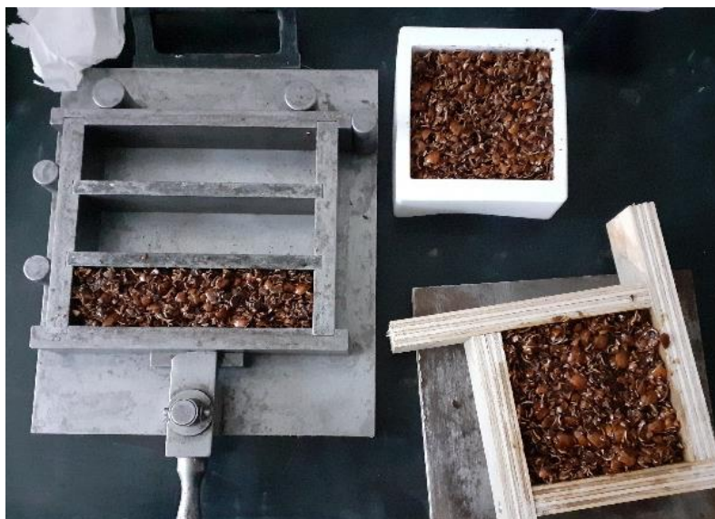
Figure 4.2-3. The considered moulds to produce the samples: metal, wooden and silicone.
