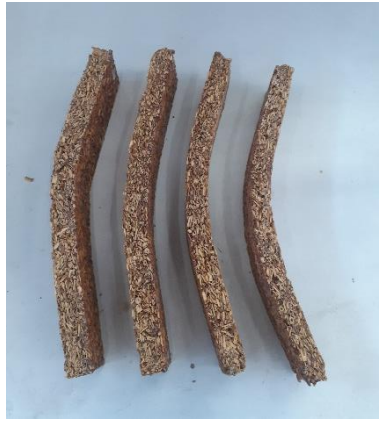
Figure 4.4-7. Four samples (10 cm x 50 cm x 4 cm) of giant reed and sodium silicate solution after the bending test.
