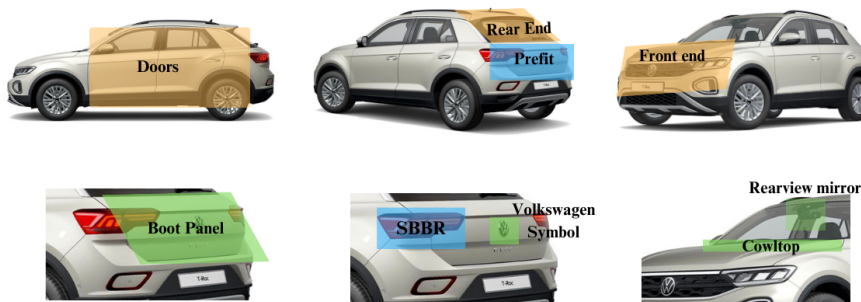
Figure 4.1: Parts of the vehicle involved in the analyzed tasks of each workstation. Blue: H 1 ; Orange: H 2 ; Green: H 3 .
