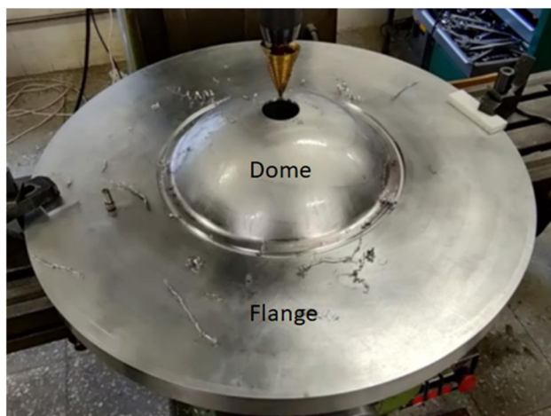
Fig. 4 Preform with the final dome profile
