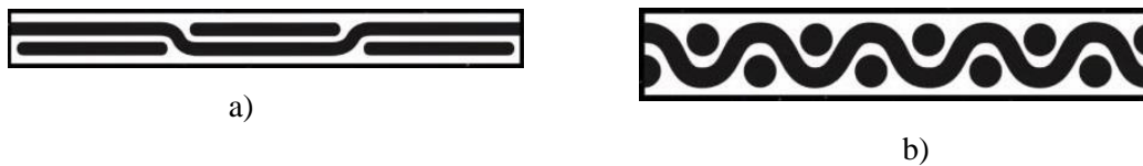
Figure 2.6 - Representative cross-section of: a) plain weave with spread tows; b) plane weave with regular tows
