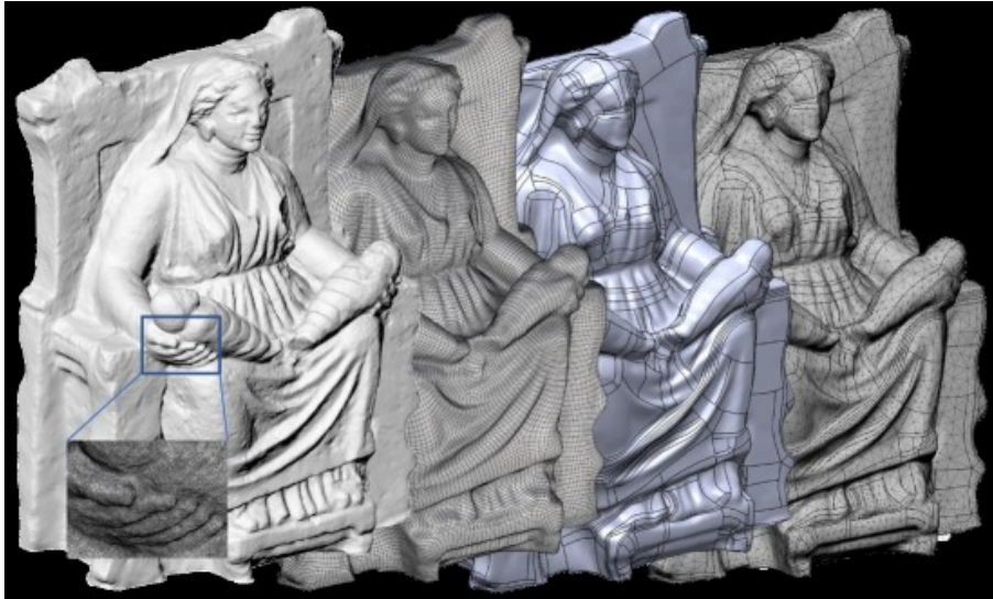
Figure 3.5: From the very dense scanned and tessellated model to the FE (Finite Element) mesh model, passing through the quad mesh and the surface model (from left to right) [24].
