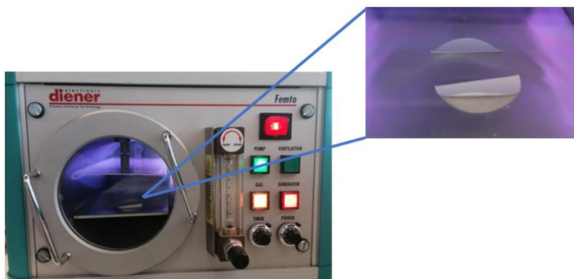
Figure 6 -Functionalization of cellulose membranes with plasma (argon gas).
