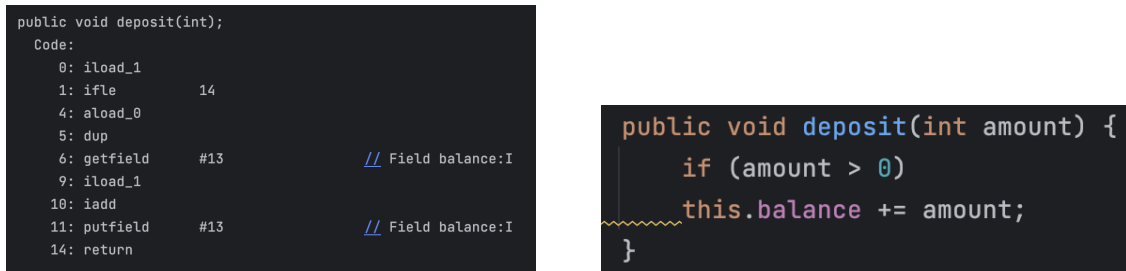
Figure 6.1: ByteCode instruction comparison to Java source code.
