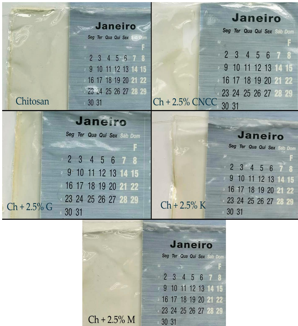
Figure 5.3 - Ch film and Ch bionanocomposites with 2.5 % CNC optical configuration. Chitosan (Ch); Commercial Nanocellulose (CNCC); Giant Reed Nanocellulose (G); Kenaf Nanocellulose (K); Miscanthus Nanocellulose (M).
