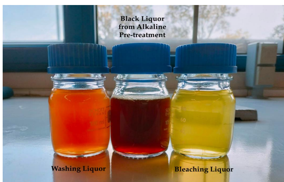
Figure 4.2 — The three residual liquors generation during the cellulose isolation.
