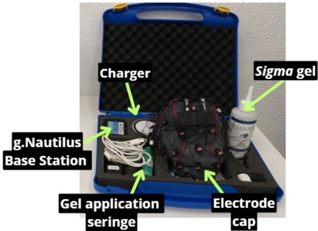
Figure B.2: g.Nautilus ® equipment for Electroencephalogram (EEG) acquisition, adapted from [20].
