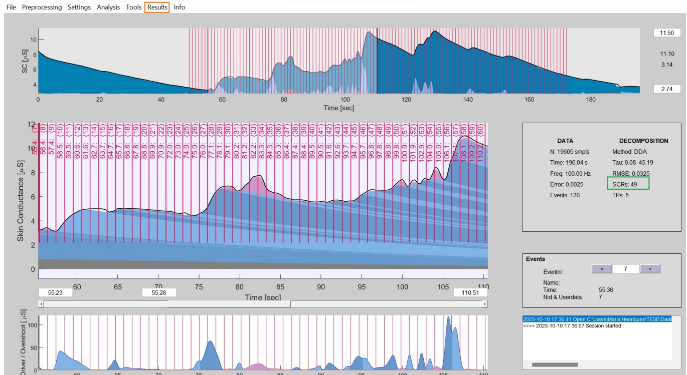
Figure 4.5: Ledalab ® software after DDA process. The top graphic shows the complete EDA signal, the middle one displays the tonic component, and the bottom one exhibits the phasic component. The red lines represent the triggers. “Results” menu and SCRs are highlighted in orange and green, respectively.
