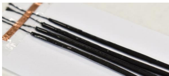
Figure 5.74 - Four cCF-Seys-TENGs connected in parallel.
