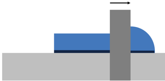
Figure A.6 — Schematic process representation of films by casting.
