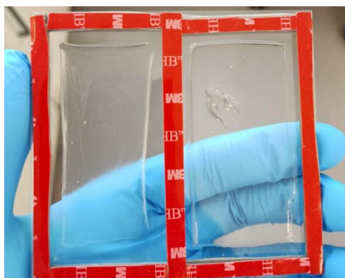
Figure 16. Example of the mould use for the fabrication of films using solvent casting method, at room temperature. The films illustrated in the photo are agarose film (AG) and agarose/borax film (AGB).
