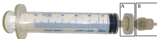
Figure 2.2: Filtration system composed by A) an pre-filter and B) a filter
