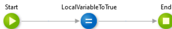
Figure 4.3 – Service Studio representation of a simple Server Action . Notice the Start and End buttons with a full green background.
