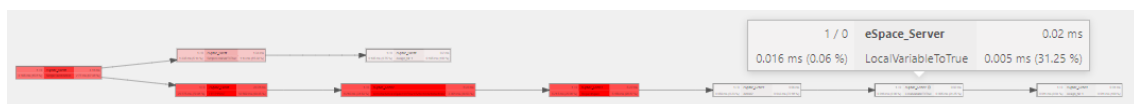
(a) Complete graph representation. The detail for span LocalVariableToTrue is open. As it is represented in a light hue (nearly white), one can infer that its time consumption is low.
