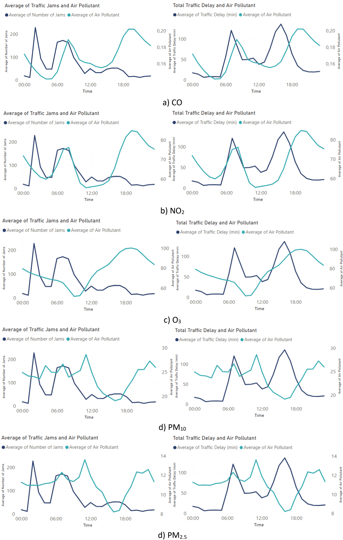
Figure 5.13 – Pollutants' concentrations vs Traffic a) CO, b) NO 2 , c) O 3 , d) PM 10 , d) PM 2.5
