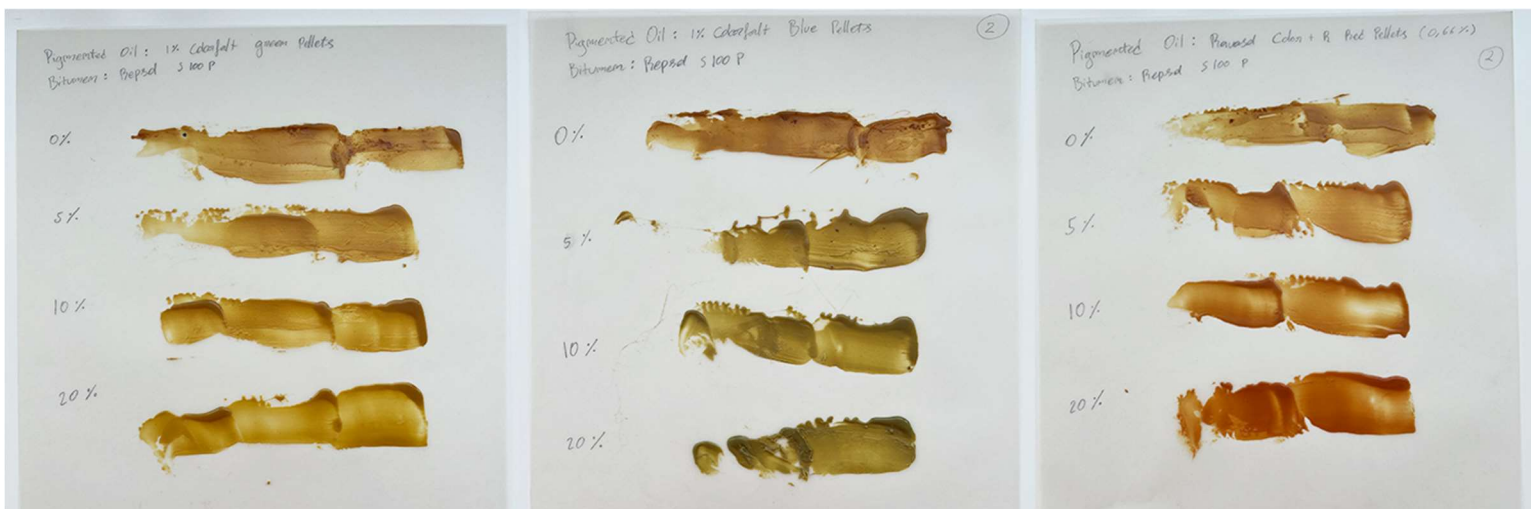
Figure 4-1: Binder pigmentation tests for sunflower oil with (left to right) 1% Colorfalt green pellets, 1% Colorfalt blue pellets, 0.66% Ravasol Color+R red pellets
