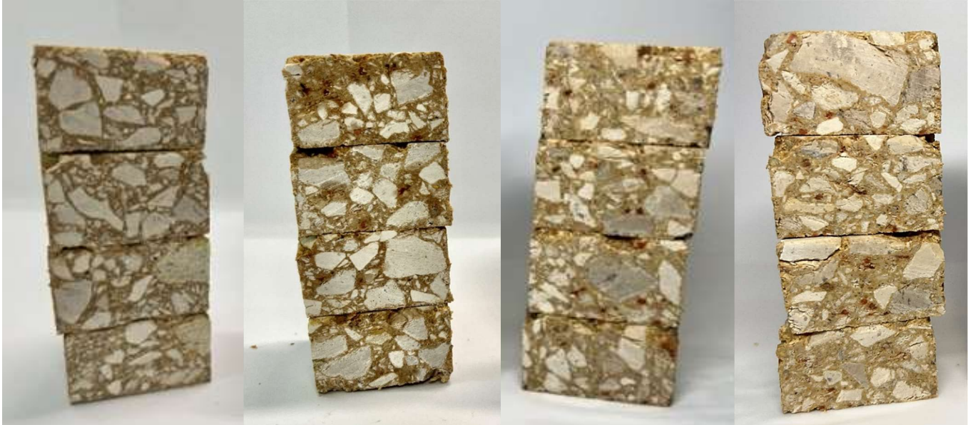
Figure 4-8: Internal structure of the cylindrical asphalt concrete specimens containing (left to right) no capsules, 0.75% capsules, 1.25% capsules, and 2% capsules
