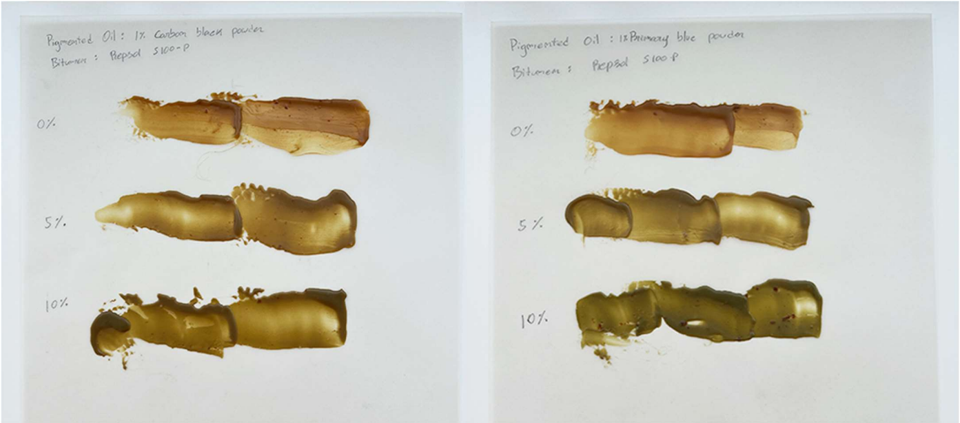
Figure 4-2: Binder pigmentation tests for sunflower oil with 1% carbon black pigment (left) and 1% primary blue pigment (right)
