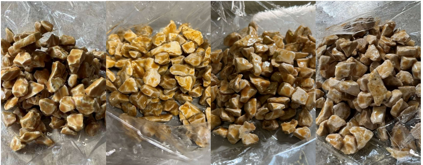
Figure 4-29: Photographs of the synthetic binder-covered aggregate after (left to right) 0, 6, 24, and 48 hours in oil
