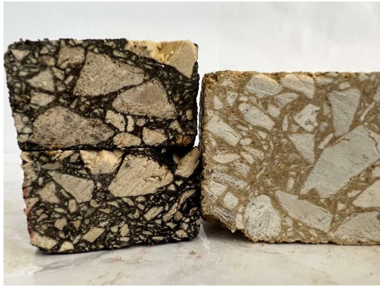
Figure 4-6: Comparison between the internal structure of limestone converted asphalt concrete mixture made with 35/50 bitumen (left) and synthetic binder (right)
