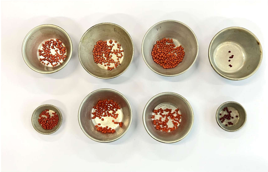
Figure 4-5: Calcium alginate capsules after being heated (top) compared to unheated ones (bottom)
