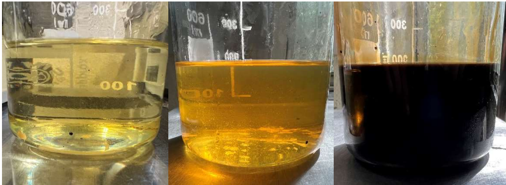
Figure 4-30: Sunflower seed oil before the experiment (left), after 48 hours in contact with the synthetic binder mixture (center), and after 48 hours in contact with the bitumen mixture (right)
