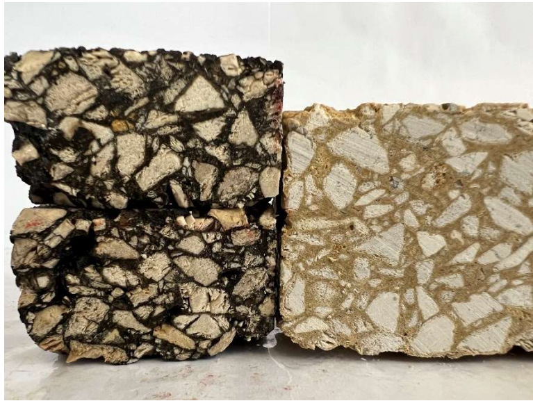
Figure 4-7: Comparison between the internal structure of limestone converted stone mastic asphalt mixture made with 35/50 bitumen (left) and synthetic binder (right)
