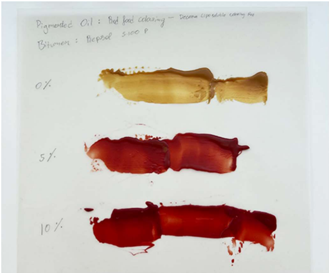
Figure 4-3: Binder pigmentation test for sunflower oil with 50% red fat-soluble food coloring
