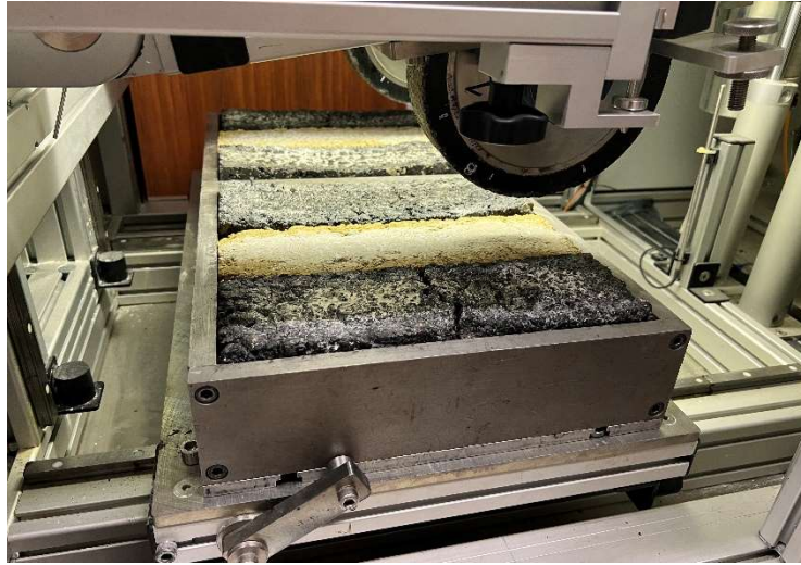
Figure 3-6: Wheel tracking simulator configuration
