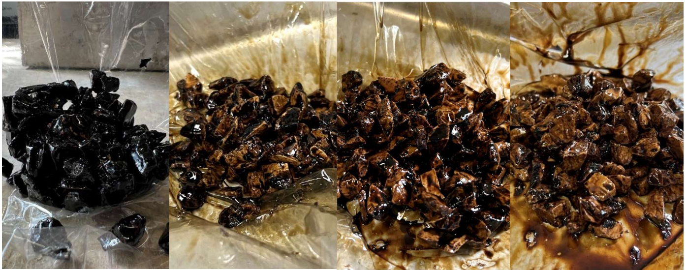
Figure 4-28: Photographs of the bitumen-covered aggregate after (left to right) 0, 6, 24, and 48 hours in oil
