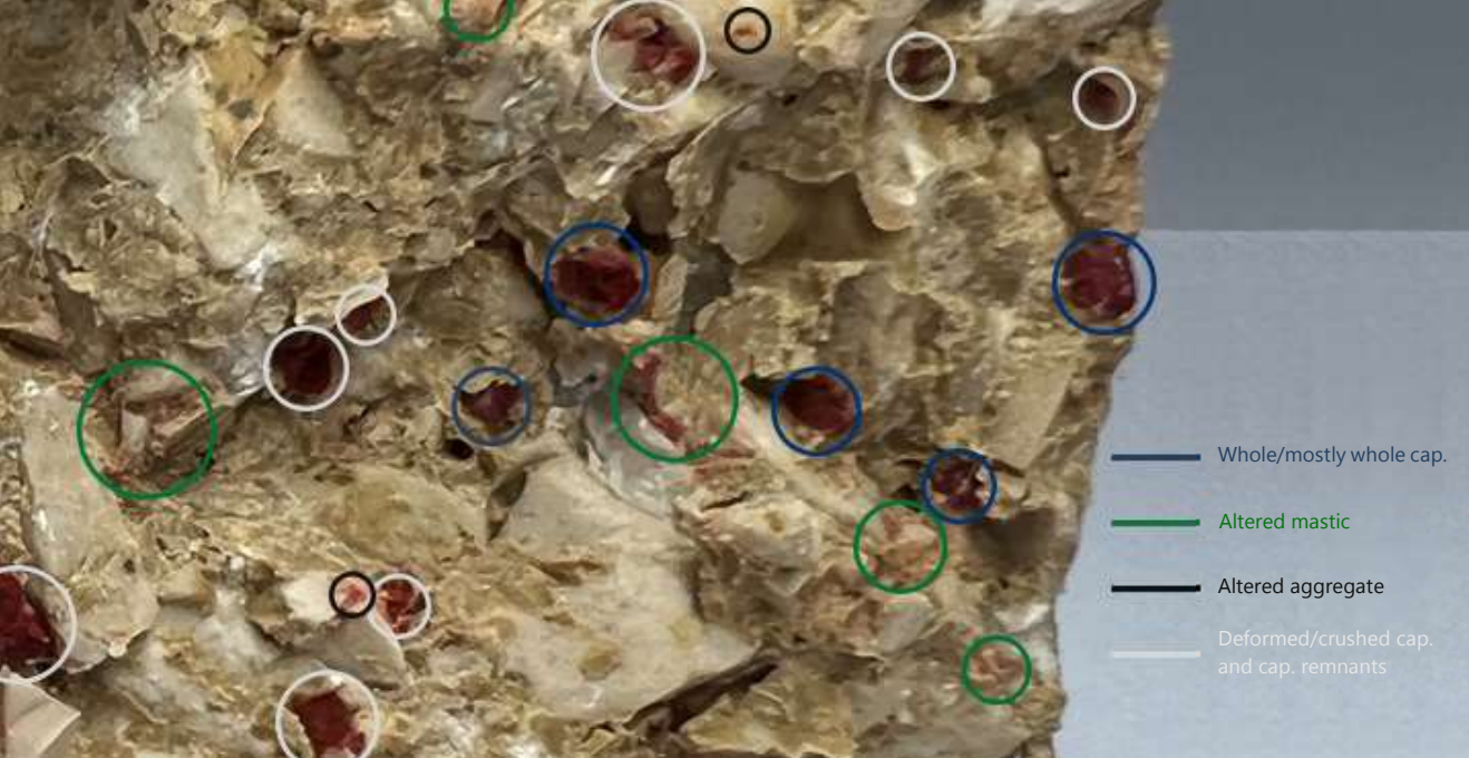
Figure 3-8: Example of the visual criteria used to identify the capsule-related occurrences
