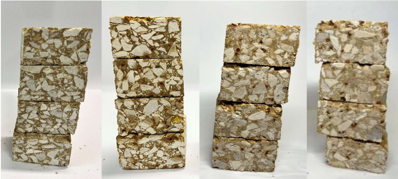
Figure 4-9: Internal structure of the cylindrical stone mastic asphalt specimens containing (left to right) no capsules, 0.75% capsules, 1.25% capsules, and 2% capsules
