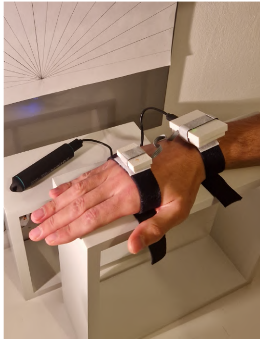
Figure 4.3: Wearable motion-sensing prototype in a final phase
