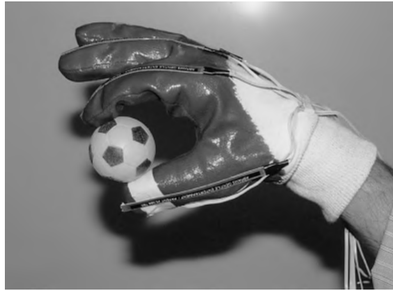
Figure 2.19: Data glove with force sensor and flex sensors [58]
