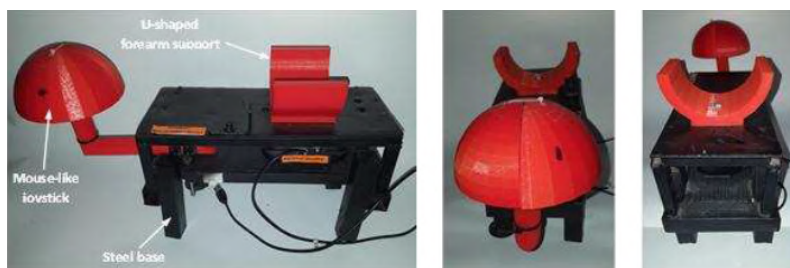
Figure 2.14: Overview of the mouse-like joystick wrist rehabilitation system [3]
