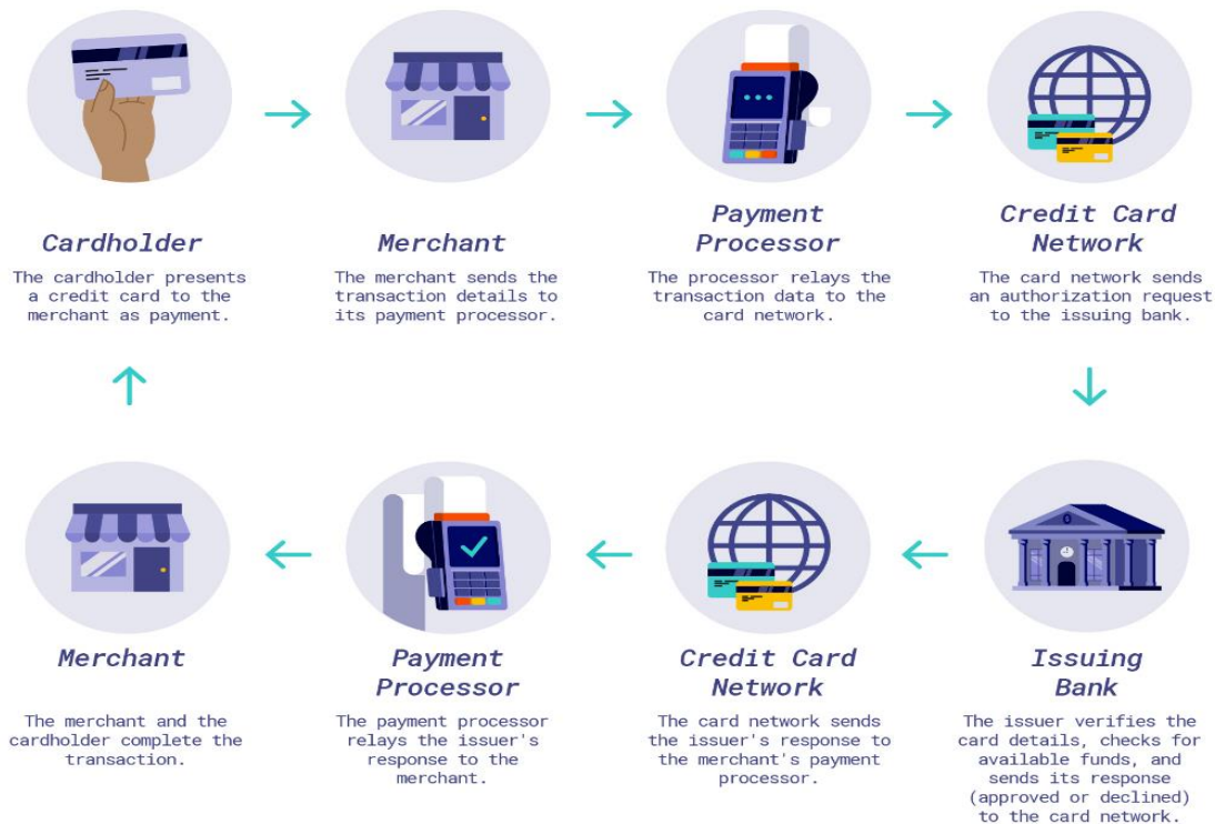
Figure 1: Steps of a payment transaction process on a POS terminal - authorization
