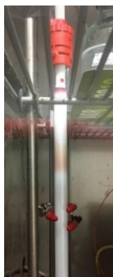
Figure 4.10 - Image of size exclusion chromatography column purifying the RIC protein.
