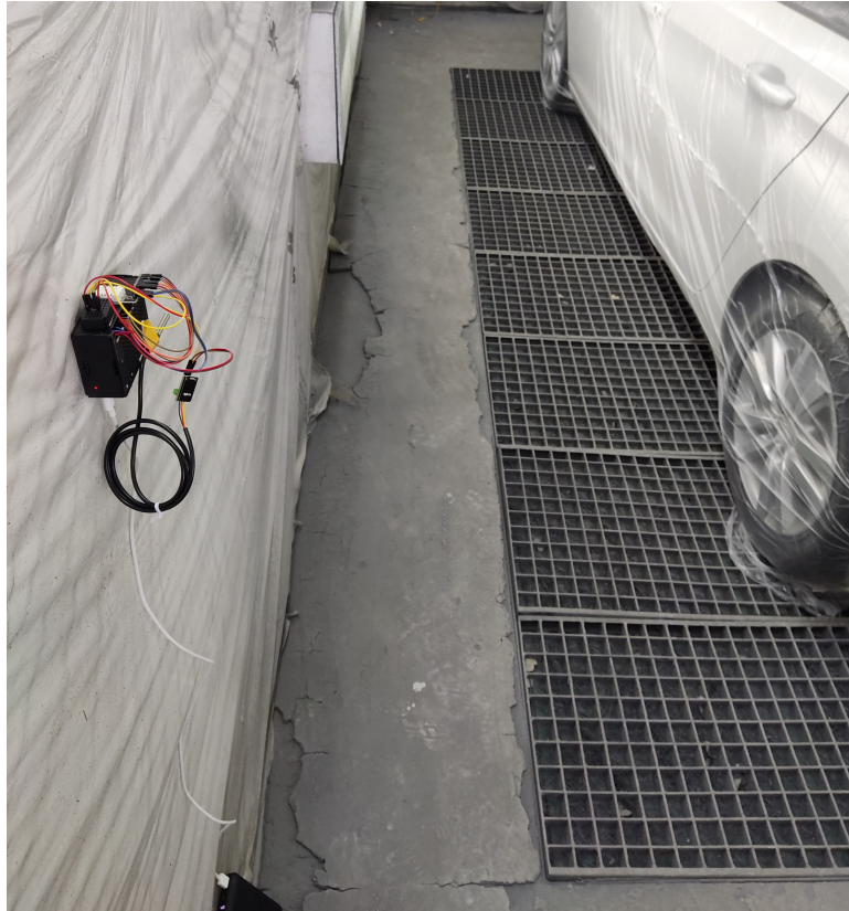
Figure 5.4: The sensor box recording temperature and humidity data inside the paint booth.
