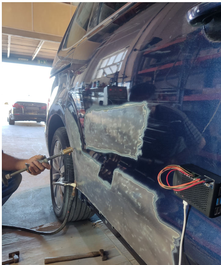
Figure 5.20: Worker using the spot welder dent puller.
