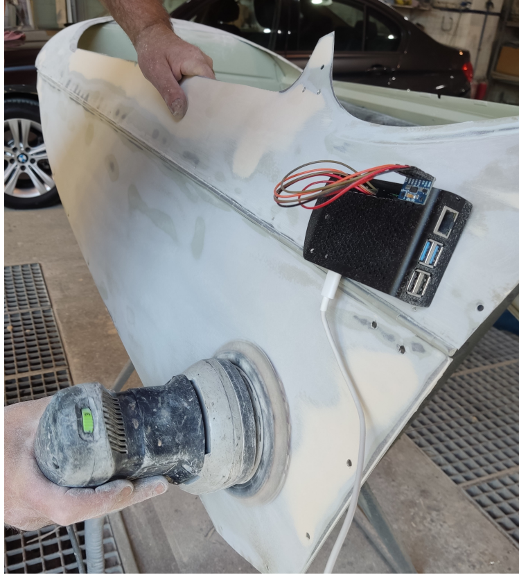
Figure 5.22: Worker using an electric sander to fix the body of a Messerschmitt KR200.
