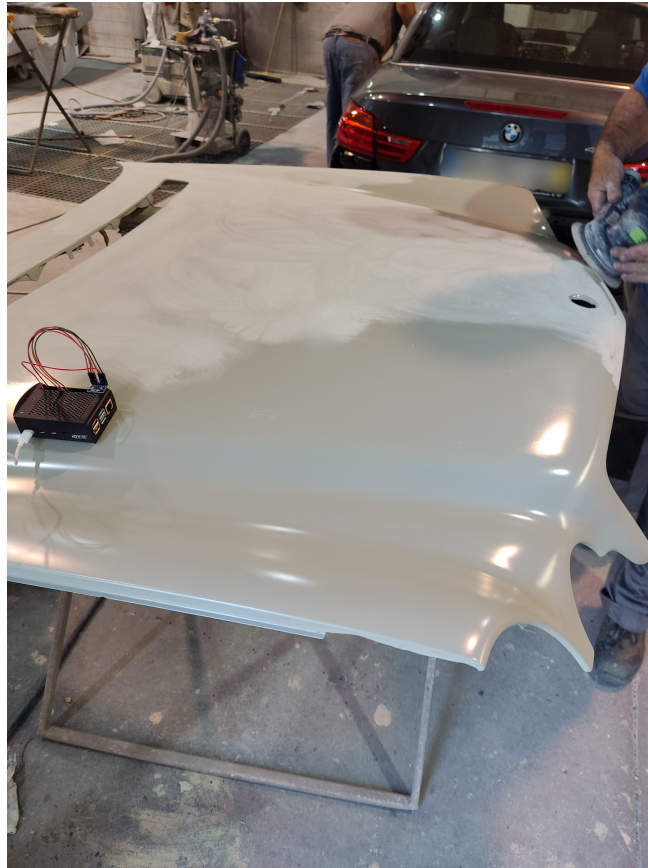
Figure 5.6: Worker using an electric sander on a Mercedes E 270 bonnet with the BMW 425d in the background.
