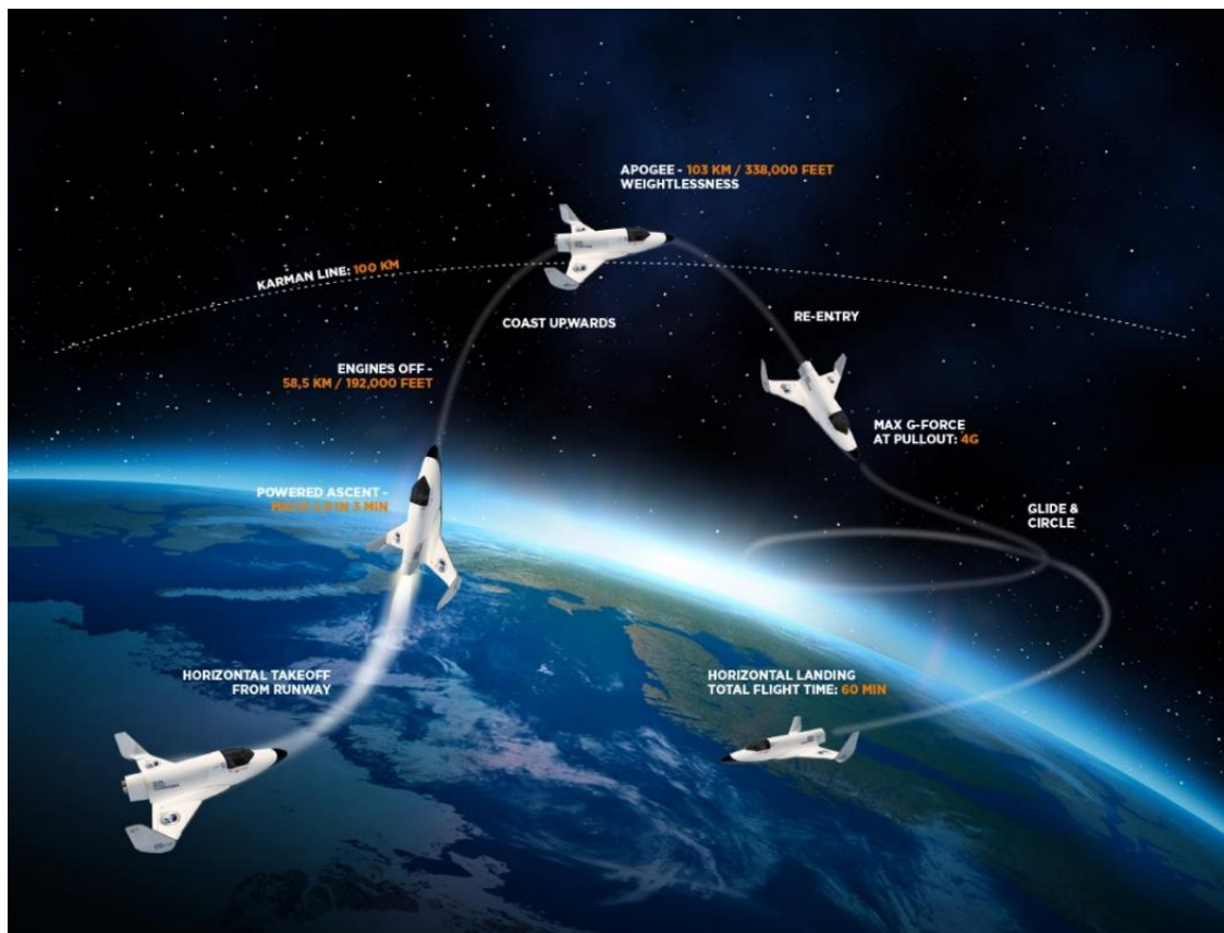
Exhibit 4: Lynx Mk. II Flight Profile (XCOR Aerospace n.d.)
